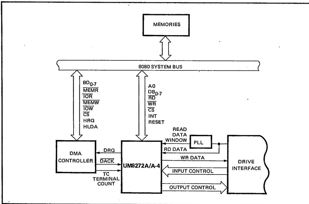
Figure 1. System Configuration
