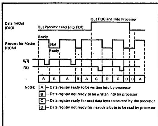
Figure 3. Status Register Timing
